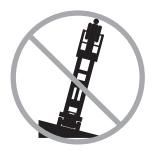
Do not depend on the tilt alarm as a level indicator. The tilt alarm sounds on the chassis only when the machine is on a severe slope.
